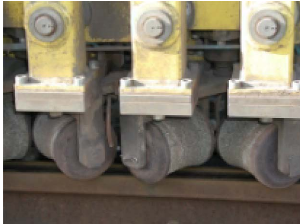
Fig. 9. Grinding stones of the prototype developed by Stahlberg-Rönsch.
