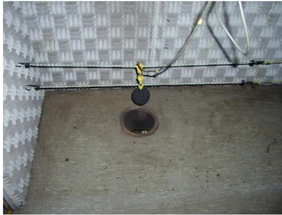
Fig. 3. Semi-anechoic microphone room inside the noise monitoring car (“Schallmesswagen”—SMW) built by DB for monitoring the sound emission of BÜG track.
